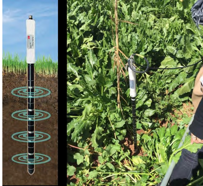
Installation des sondes capacitive
